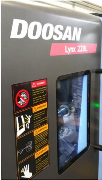
machines have a work envelope of 23.3 x 22 x 23.3 and 14k spindle.
